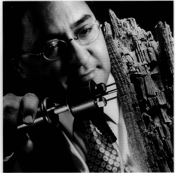
Fig. 2. The author using a hammer probe to measure the deep moisture content of timber.
